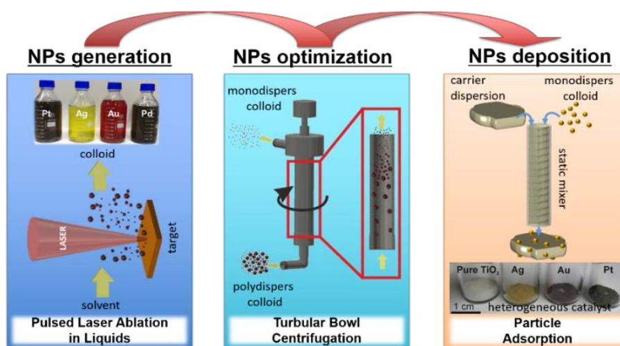
Figure 1: Schematically scheme of the continuous process chain from laser-generated NPs and size selection to a heterogeneous catalyst.
