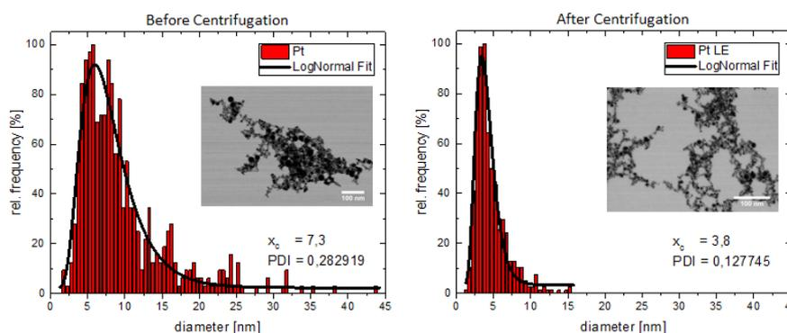
Figure 2: TEM-images and size distributions for laser-generated Pt-NPs before (left) and after (right) centrifugation in the tubular bowl centrifuge
