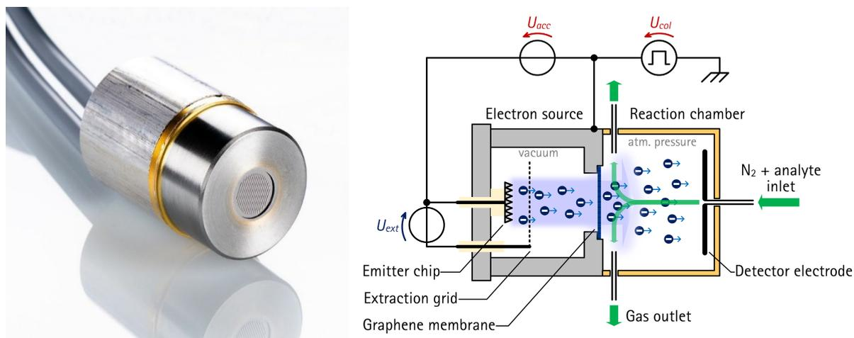
Fig. 1: Non-radioactive electron emitter based on field emission (left) [KETEK GmbH], schematic of a pulsed non-radioactive ECD (right)
