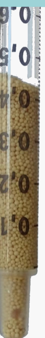
Fig 6: Resulting bed from sedimentation in a syringe
