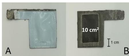
Fig. 1: photographs of Sn-based GDE. A: PTFE covered gas-site. B: electrolyte-site
