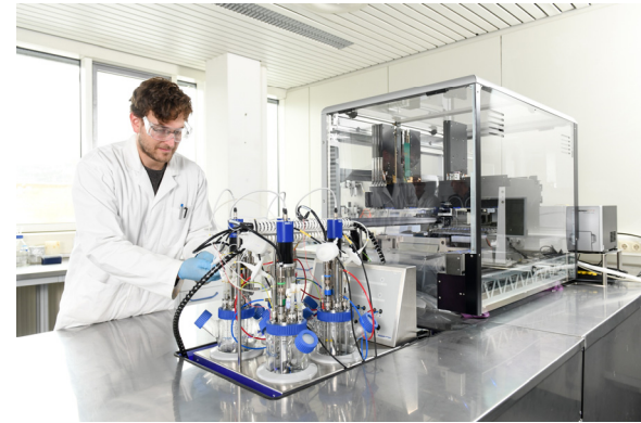
Fig. 1 – Photo of the multi-scale cascade of parallel stirred-tank bioreactors for automated bioprocess development: Up to 4 L-scale stirred-tank bioreactors can be used automatically for cell production. An automated biomass transfer system ensures the subsequent transfer and distribution of the cells into up to 48 parallel stirred-tank bioreactors on a 10 mL-scale for performing individual parallel protein expression studies automated by a liquid-handling system with integrated fluorescence reader.
