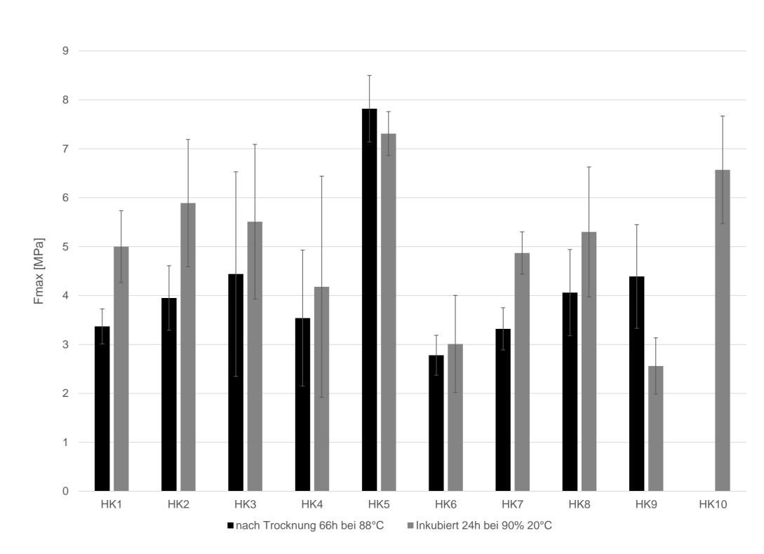
Results of adhesion force measurement of various specimens HK1-HK10; HK5 is a commercial petrochemical reference "Ponal Waterproof". Samples were dried for 66 h at 88 °C in drying oven. Then incubated for 24 h at 90% humidity and 20 °C.
